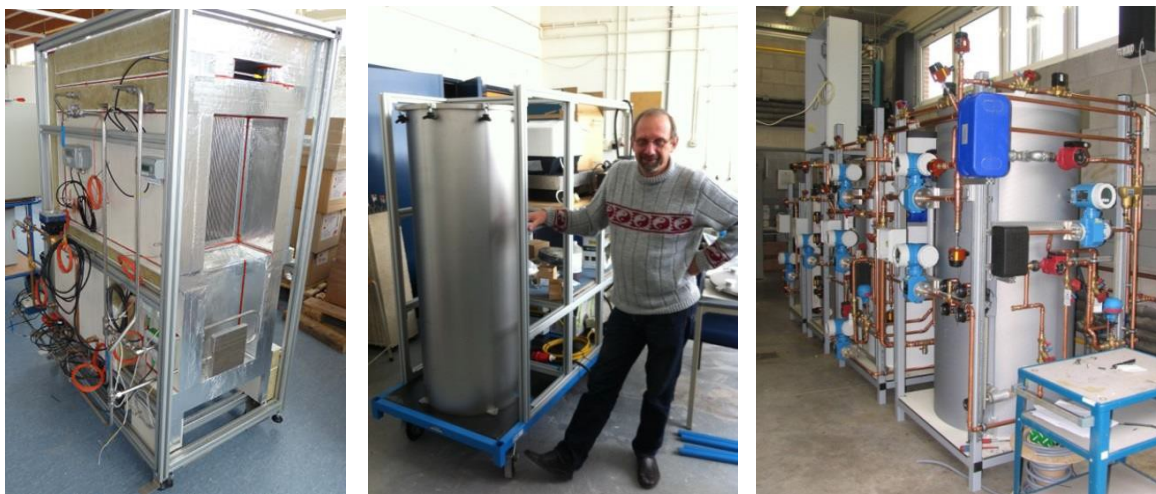
Figure 3: 14 kWh TCM reactor at ECN (left), 3 kWh TCM reactor at TNO (middle) and test rig with water vessels in the lab of VITO (right).
